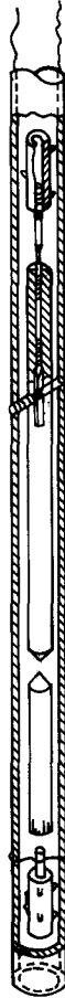
FIGURE 11. Apparatus employed by Kolm & Herlin (1956) to study the dynamics of helium II. The inner cylinder is shown suspended by Beams type of magnetic suspension. This cylinder was set into rotation and observed to coast to rest as shown in figure 12.
